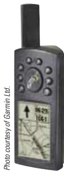
Figure P39.55 This global positioning system (GPS) receiver incorporates relativistically corrected time calculations in its analysis of signals it receives from orbiting satellites. This allows the unit to determine its position on the Earth's surface to within a few meters. If these corrections were not made, the location error would be about 1 km.
